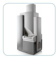
The **MALDI 4800 TOF/ TOF** (ABI Sciex) is a tandem time-of-flight MS/ MS system, providing not only peptide identification but peptide sequencing. It is also suitable for MW analysis of intact proteins.
