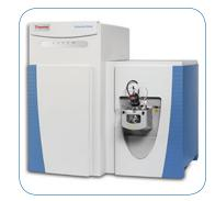
The **Q-exactive** (Thermo Fisher) is an hybrid quadrupole-Orbitrap high resolution/high mass accuracy mass spectrometer useful for untargeted or targeted screening and a broad range of qualitative and quantitative analysis.
